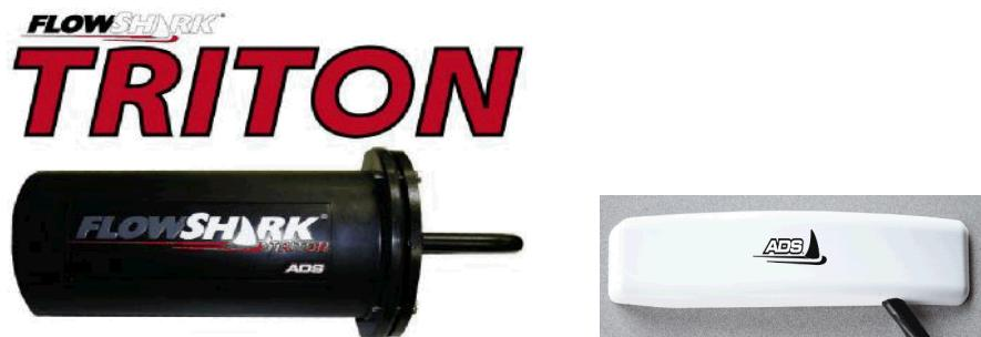
The **ADS FlowShark Triton** monitor was selected for this project. This flow monitor is an area velocity flow monitor that uses both the Continuity and Manning's equations to measure flow.
