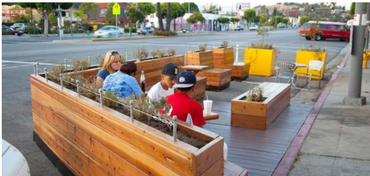
Parklets can take the place of several parking spots and serve as large curb extensions. This parklet provides public seating on Huntington Drive in El Sereno in an area where angled parking was prohibited. The space allows for sidewalk-adjacent dining (LADOT People St Flickr Photostream).
