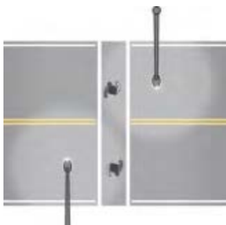
Overhead Crosswalk Illumination Placement
