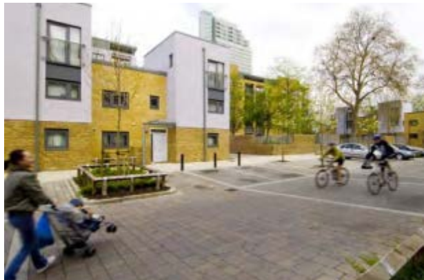
This street uses textured pavers, street trees, and parking to invite play and slow speeds.
