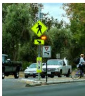
Rectangular Rapid Flash Beacon at an Uncontrolled Crossing (Lara Justine, Flickr CC)
