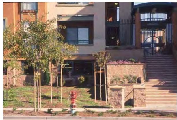
Exposed podiums should include detailing and design such as concrete blocks with special surface textures.
