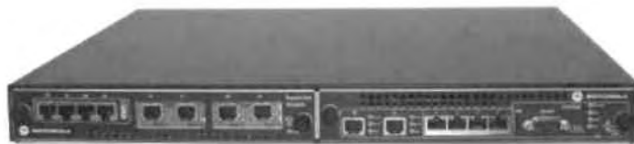
Figure 1-3: Enhanced GGM 8000 Conventional Channel Gateway - Connects dispatch operators to analog or digital conventional channels in the system.
