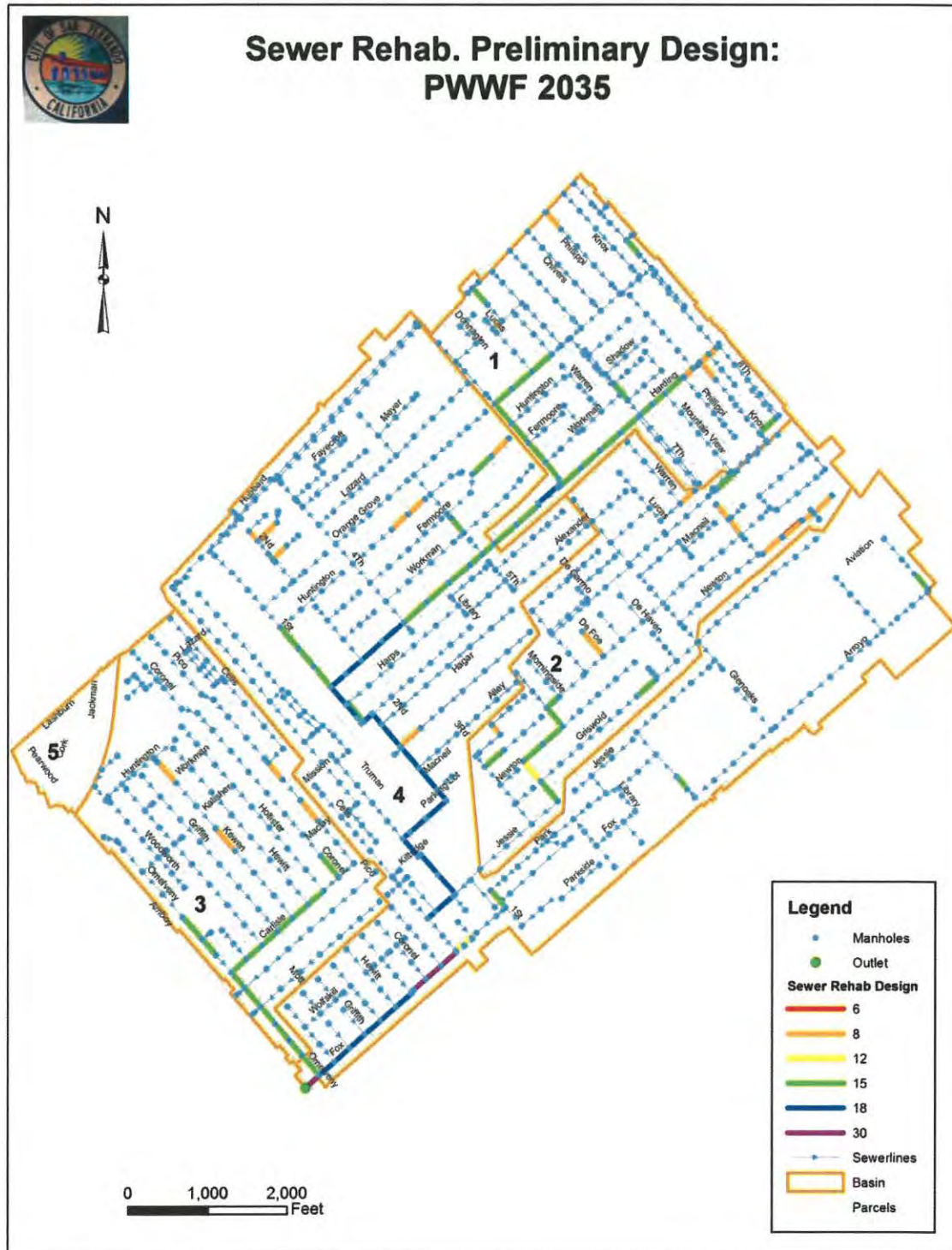
Figure 6-3 – Sewer Rehabilitation Preliminary Design
